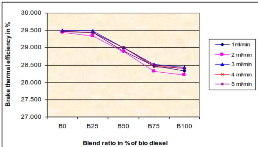
Figure 4. Brake Thermal Efficiency vs Blend Ratio
