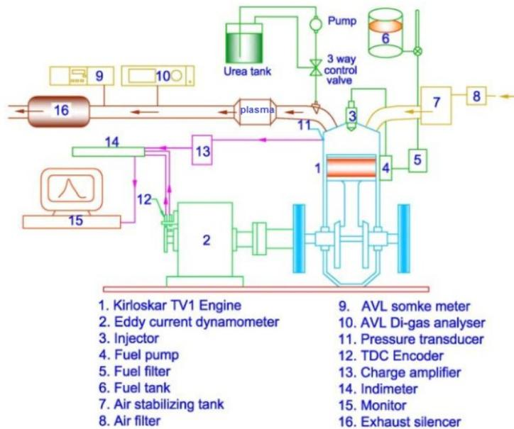
Figure 1. Schematic diagram of the engine test setup
