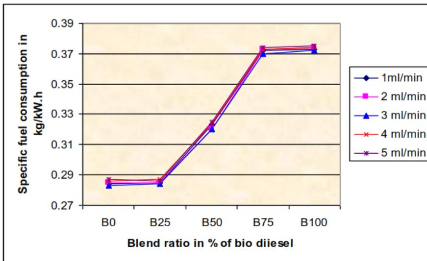
Figure 3. Specific fuel consumption vs Blend ratio
