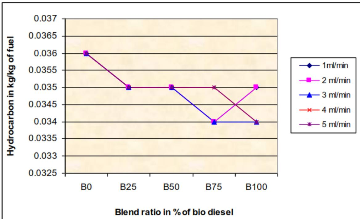
Figure 9 Hydrocarbon vs Blend Ratio
