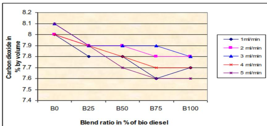
Figure 7. Carbon dioxide vs Blend Ratio
