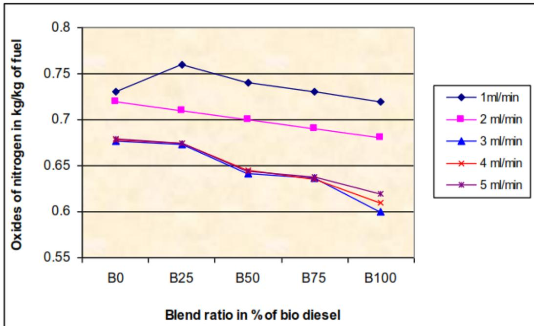
Figure10 Oxides of Nitrogen vs Blend Ratio
