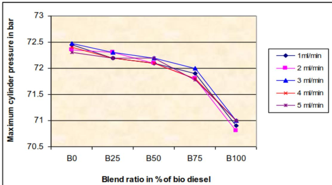
Figure6.Maximum Cylinder Pressure vs Blend Ratio
