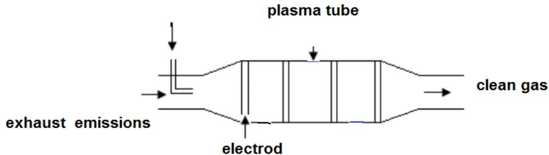
Figure 2. Schematic diagram of the plasma setup
