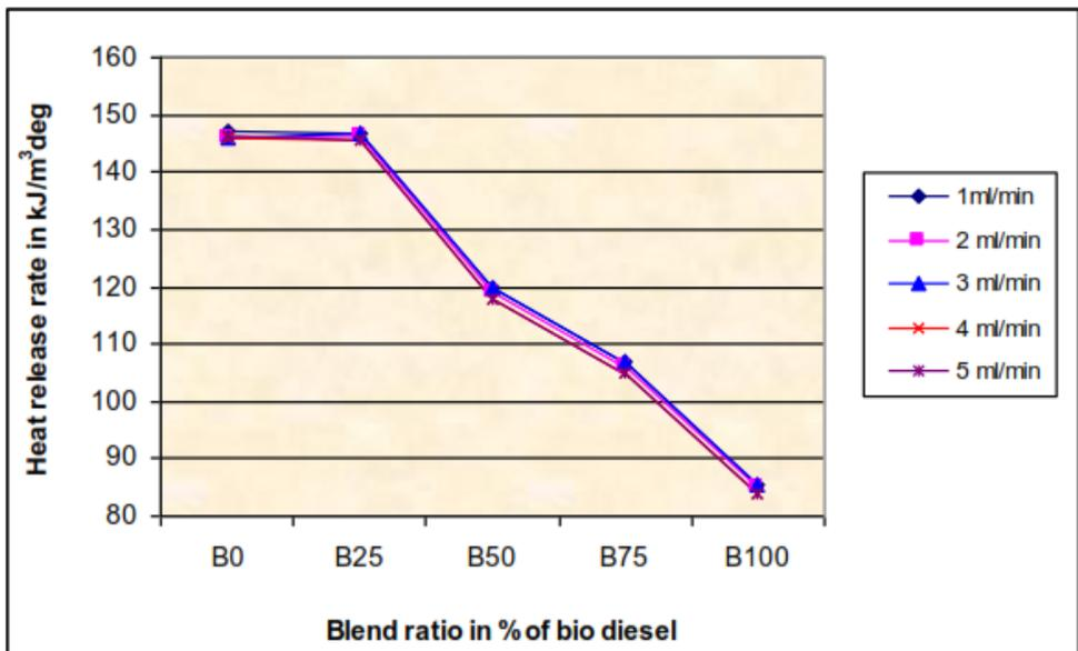
Figure 5. Heat Release Rate vs Blend Ratio
