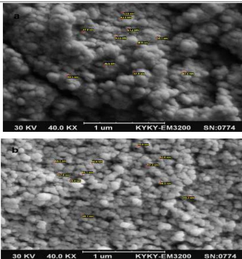
Fig1. SEM image of nanoparticles (a) MgNiFe2O4 and (b) PdNiFe2O4.
