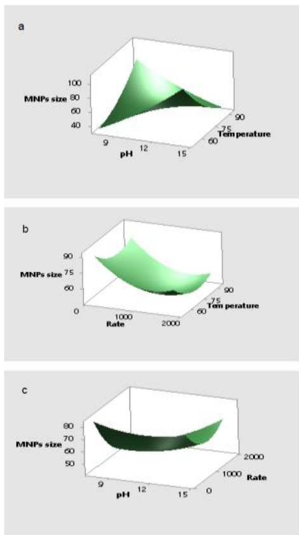
**Fig.6.** Response surface plots representing the effect of three variables: reaction (a) rate to temperature. (b) reaction rate to pH and (c) pH to temperature.
